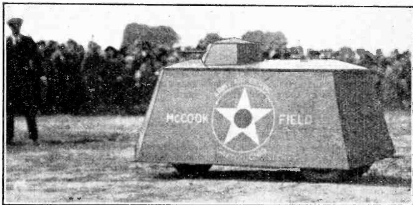
WIRELESS WAR OF THE FUTURE. A wireless-controlled tank photographed under test at Dayton, Ohio. This unusual form of weapon is being developed by the U.S. Army Air Service.
